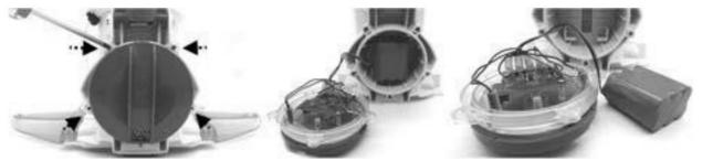
2. Disconnect the battery cable by pressing the connector clip and pulling it out.
