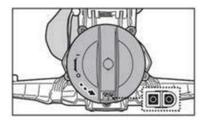
2. Connect the charging plug to the charging port. **WARNING!**Do not reverse the polarity of the charging plug and make sure the charging plug and charging port are clean and dry before charging. TIPS: Use a cotton swab to dry the charging port and charging pins. Plug the charging cable of the external power source into the charging plug.
