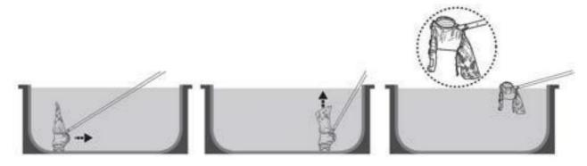
Once the pool cleaner is out of the water, the impeller will stop rotating after 2-3 seconds. The LED indicator will turn blue. When the battery charge level drops, the blue indicator will flash.
