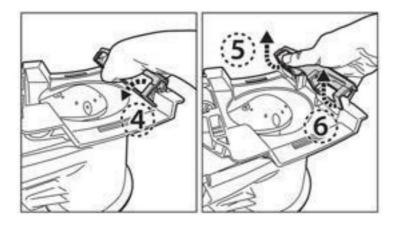
Before removing the damaged front wheels, you must first dismantle the frame.
